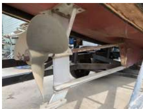
22X32 Propeller w/ stainless steel skeg and rudder support
